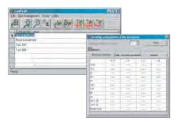
**CptBSoft and CptASoft** have been developed to program the parameters and read in real-time mode the variables of the compact power transducer (Basic and Advanced version respectively). The CPT transducers are equipped with an auxiliary serial port (RJ12 connection) in order to easily configure all the models.
